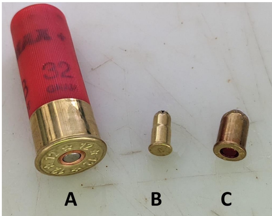
Figure 5. Consumables required for firearms or captive bolt tools. A = 12 gauge shotgun (Falcon 1200 Trap Cartridge, c. 70 cents ea.), B = Jarvis PAS 0.25R captive bolt tool (black activator – 260 mg charge, c. 35 cents ea.), C = Blitz-Kerner captive bolt tool (blue or red activator – 410/460 mg charge, c. $1.50 ea.).
